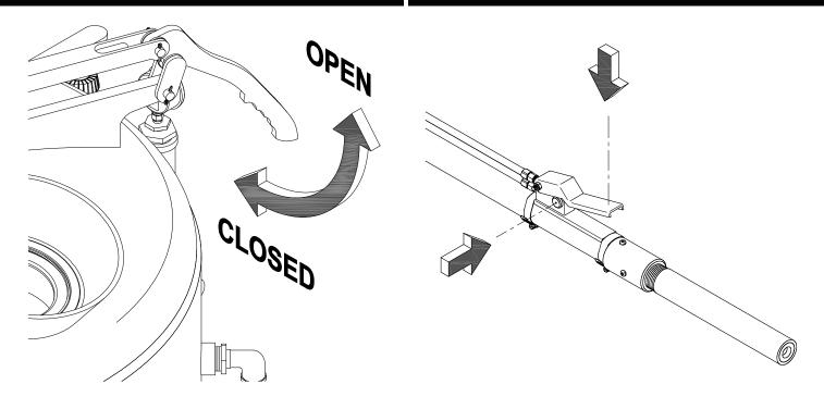
To stop blasting, let go of deadman. To shut down, close air inlet valve, open blow down valve.
