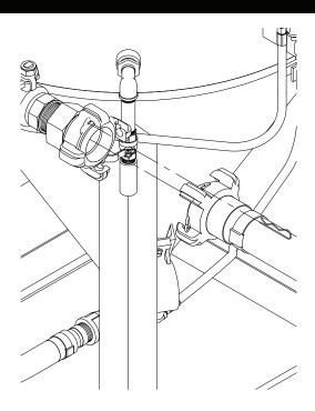
5. Fill machine with water until it pours through overflow. Close overflow.
